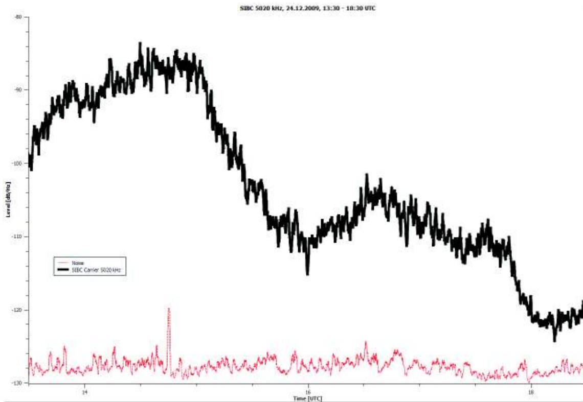
Figure 21: The reception of SIBC Honiara on December 24, 2009 at 1500 UTC shows the optimum reception time.
